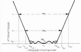
fig. A-1. A typical attenuation versus frequency response of a bandpass filter includes the parameters defined in *Appendix A*.
